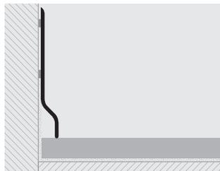
1: Choose the skirting in the required the colour. 2: Lay the skirting using quick-setting acrylic silicone, mastic or bostik, suitable for gluing flexible PVC onto mortar-plaster-accessorised walls, etc. or fix with screws/nails.
