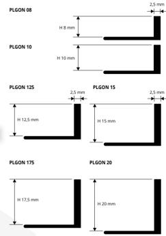
**PROLEVIGAL** are separating profiles used to create the technical joint in the special types of pavements such as marble- Venice- palladium ones, that must be smoothed after their laying process. The particular "L" shape with the cut/drilled base and 2,5 mm thick vertical edge consent the perfect smoothing and constant thickness as well. Available in natural aluminium and natural brass, various thickness, as well in outlined/bent **PROLEVIGAL** CURVE AL versions.
