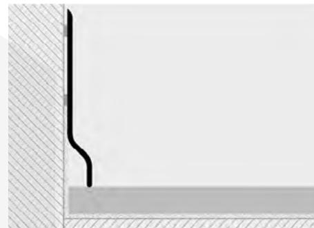
1. Choose the "SKIRTING" in the required colour. 2. Lay the "SKIRTING" using quick-setting acrylic silicone, mastic or bostik, suitable for gluing flexible PVC onto mortar-plaster-accessorised walls, etc. or fix with screws/nails.
