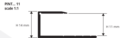
ALUMINIUM COVERED (80 wooden finishes of which 70 on demand) thermo packed - bar length 2,7 lm - pack. 20 Pcs - 54 lm (H 11 - H 15 mm - 80 lm)
