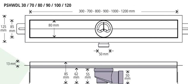
CORPO DA CONDUTA EM AÇO INOXIDÁVEL AISI 304
